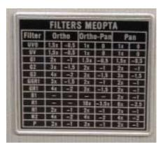
The backside of the camera has a filter compensation guide.
